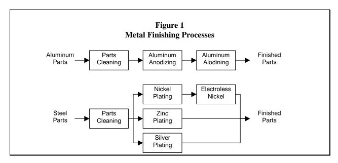
In addition to rinse waters, spent process baths are also a source of waste generation. As contaminants build up in the baths, they become unusable and must be replaced.
